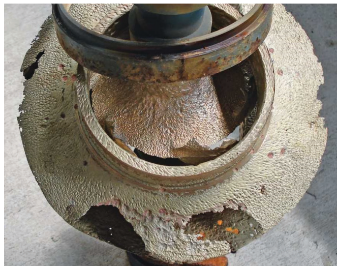
Image 2. Worn and corroded bronze impeller.
