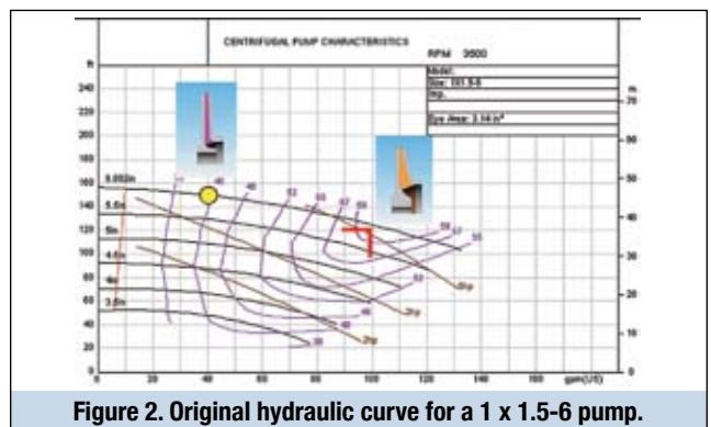
the impeller eye. This recirculation cavitation damage increases the farther away from the BEP that the pump operates.
