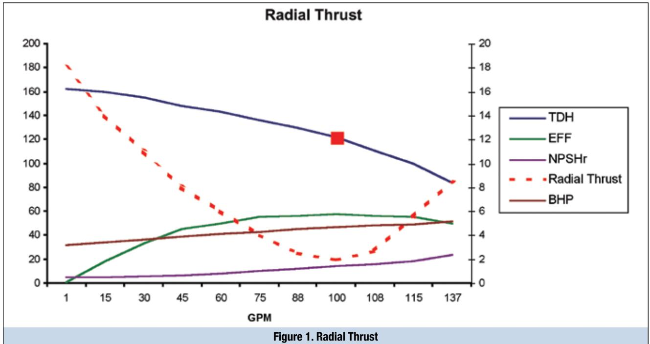
the operational cost (maintenance cost plus the cost of energy). The larger the pump, the more energy is wasted when a pump operates off the original design point.
