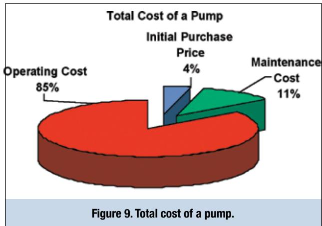
of 2000-gpm at 280-ft instead of 4000-gpm at 240-ft. The efficiency at this new point would be increased to 81 percent:  $\$145,152 \times (70/81) = \$125,440$ . The electrical savings would be:  $\$145,152 - \$125,152 = \$20,000$  per year, or about 13.8 percent in this case.
