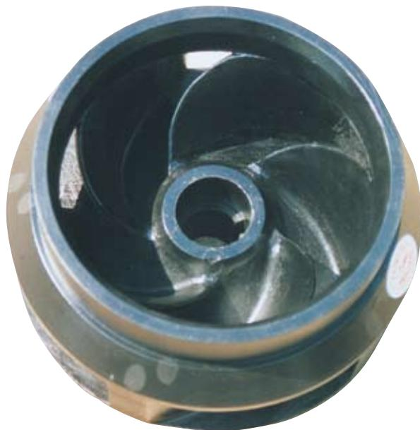
**A reengineered impeller that uses a graphite combination-fiber reinforced composite material with phenolic resin.**
