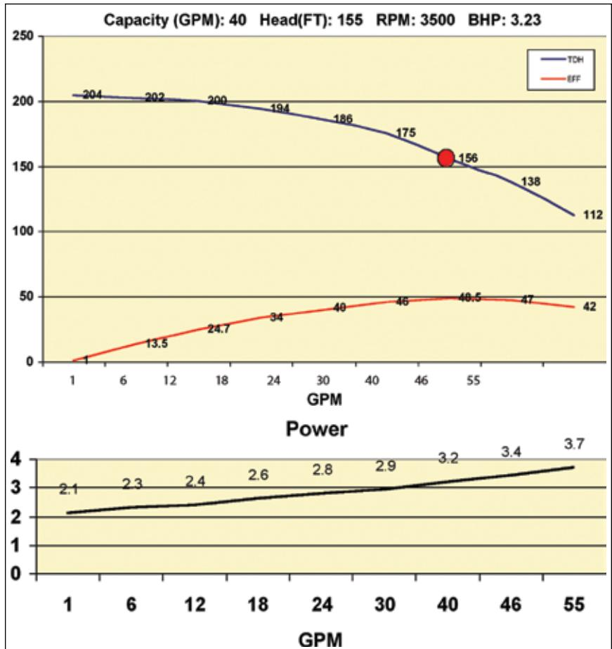
Figure 3. The performance curve of the 1 x 1.5-6 pump using a reengineered impeller.
