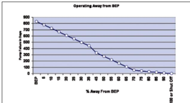
Figure 4. Operating away from the design point. This chart represents an average failure mode based on information compiled of pumps operating away from their design point.
