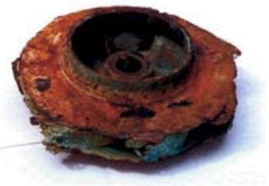
**In the case of suction recirculation cavitation (shown on the left), coatings are ineffective against cavitation damage. On the right is an example of discharge recirculation cavitation.**
