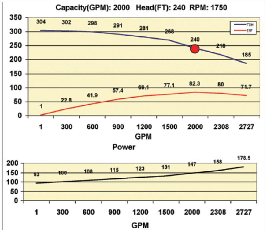
Figure 8. The performance curve of the 8 x 10-17 pump using a reengineered impeller.
