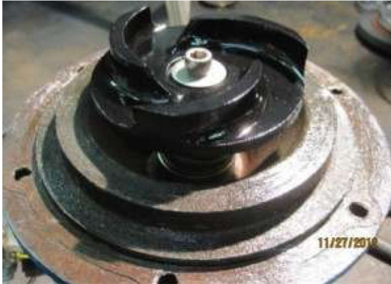
SIMSITE® Non-Clogging Impeller not clogged by the fibers
