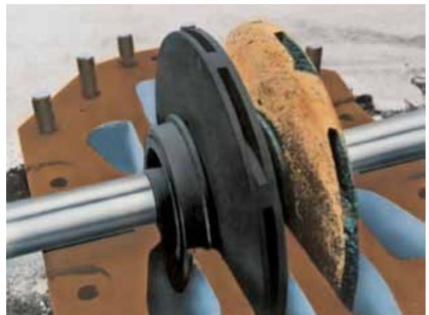
**Figure 2. Both impellers ran for three years. The structural composite impeller on the left looks like new.**
